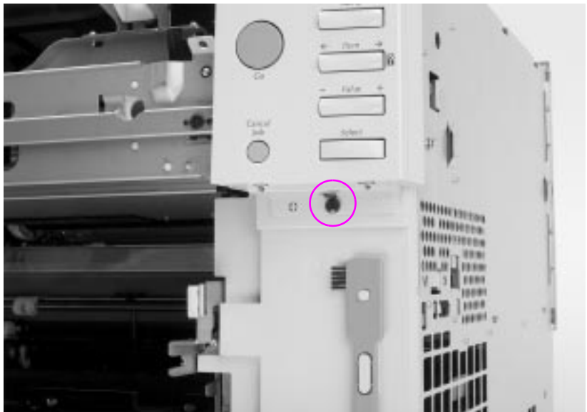
Figure 6-11 Control panel removal and replacement
